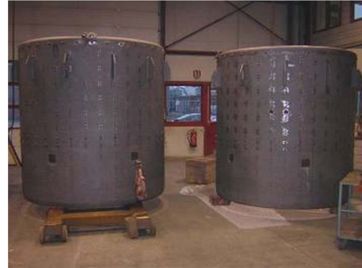
New & repair Flame tubes
