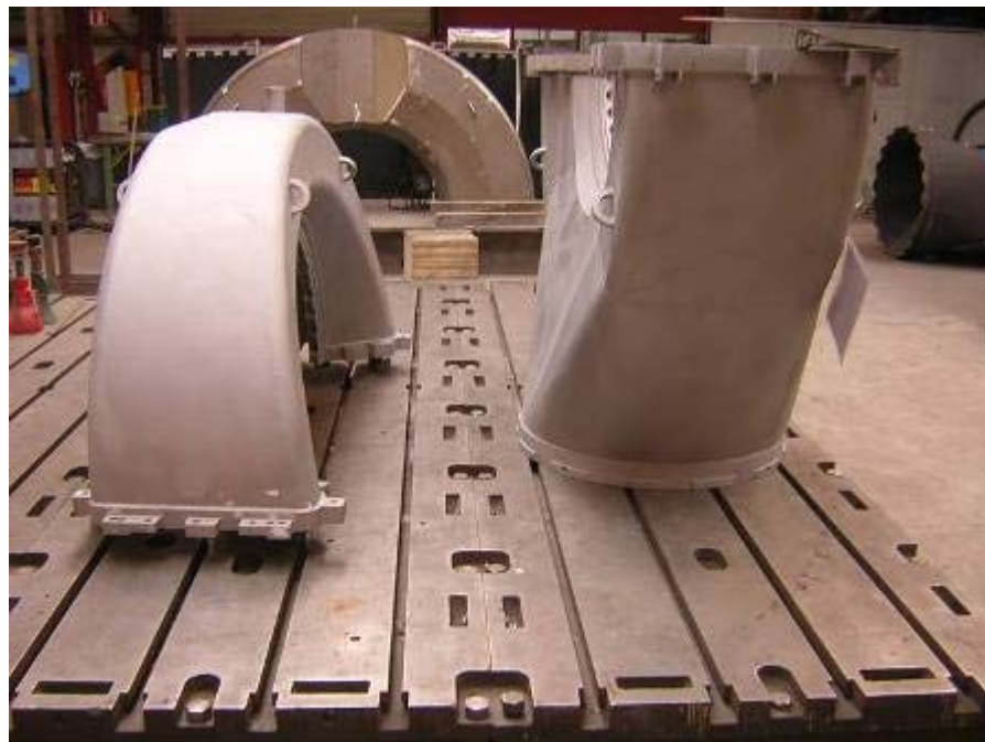
New & repair Hot Gas Casing
