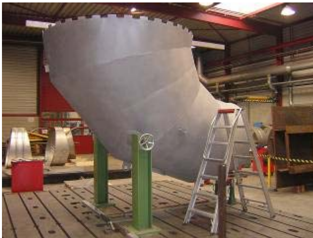
New & repair Mixing chamber
