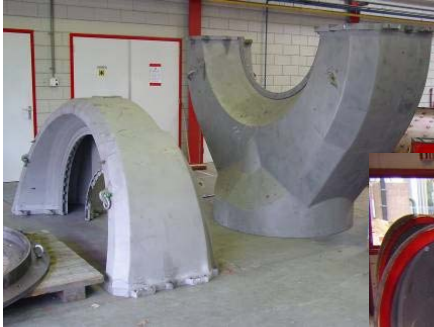
New & repair Hot Gas Casing
