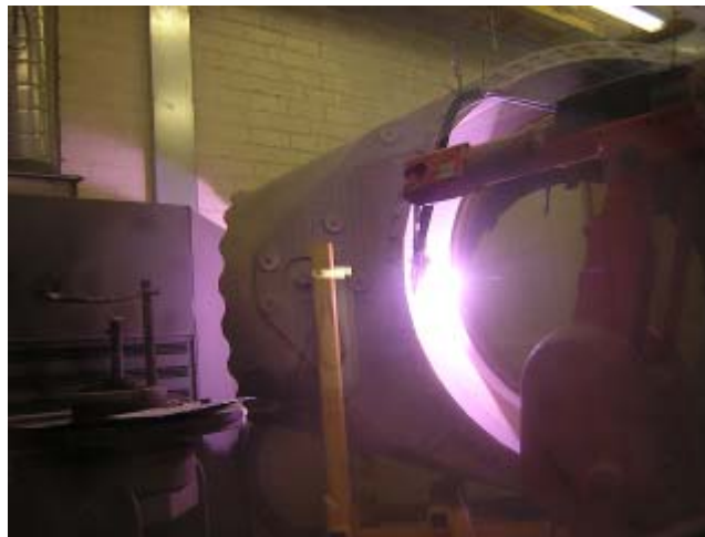
TBC coating of large combustion components
