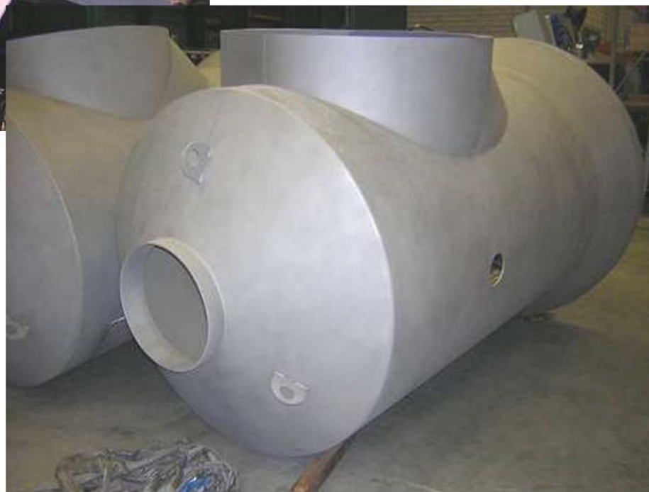
New & repair Mixing chamber
