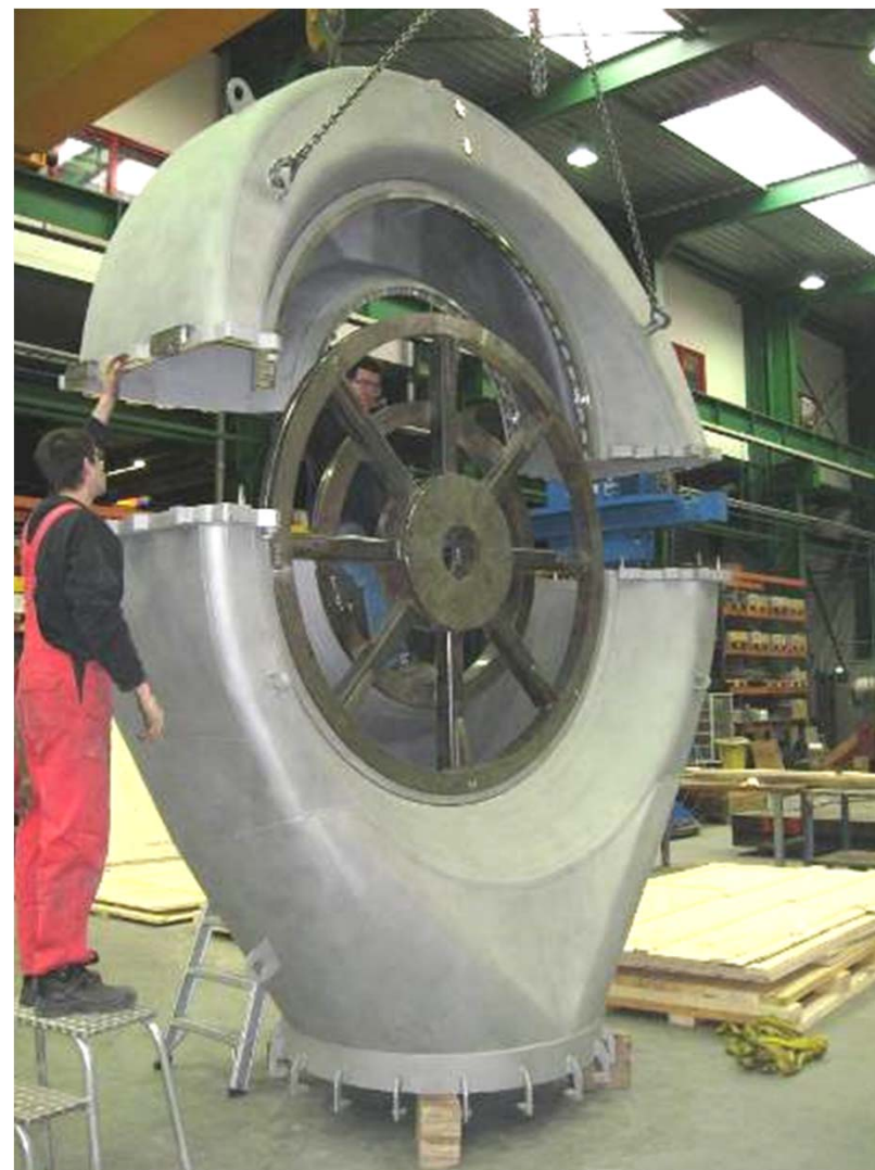
New & repair Hot Gas Casing
