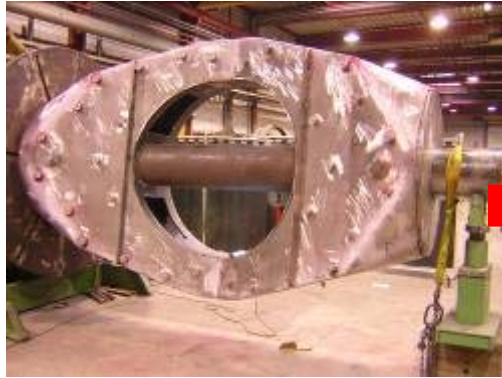
Forming of sheet metal and construction of body by welding
