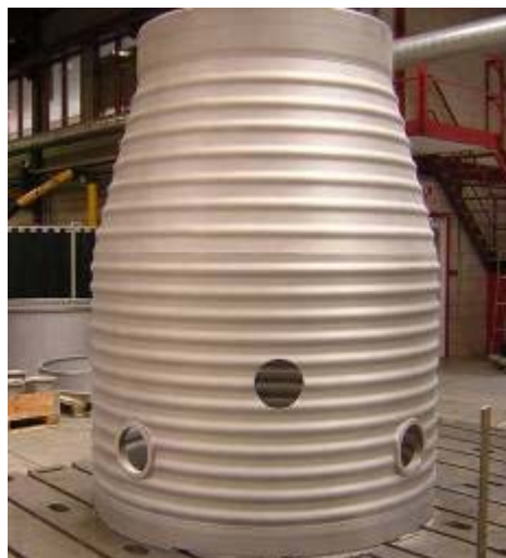
New & repair Inner Liner
