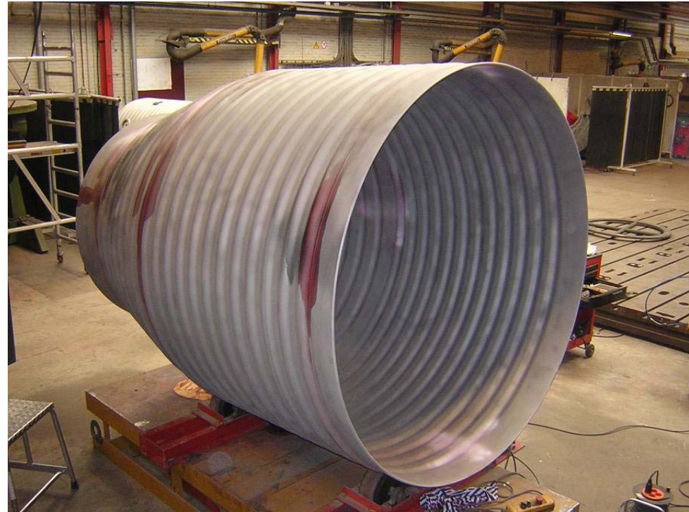
Inner liner dye check
