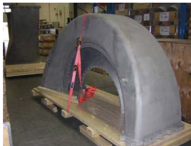
New & repair Hot Gas Casing
