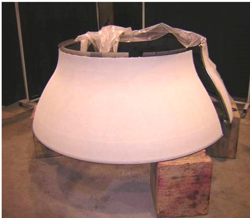
Repair Zone 2 Inner Liner
