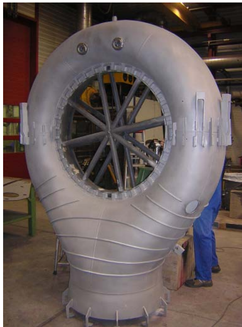
Repair Hot Gas Casing
