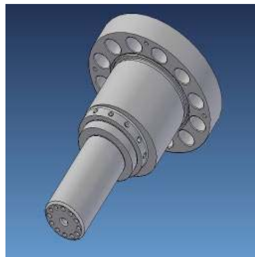
Excentric bush, excentric pen and related hardware
